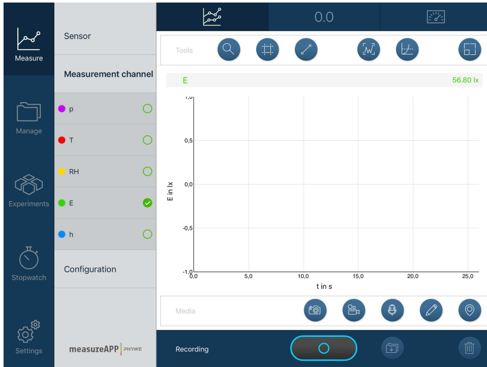
Fig. 4: Selecting the measurement channel Brightness E in the measure APP. The other parameters are not required.
