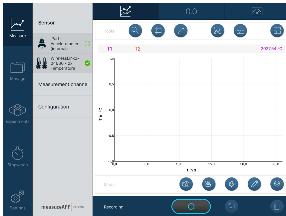
Fig. 2: Selecting the sensor Temperature
