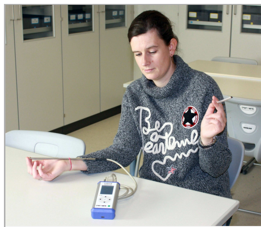
Fig. 1: Change in the skin temperature during smoking (left: measurement with Cobra4 Wireless/USB-Link for measureAPP and measureLAB, right: measurement with Cobra4 Mobile-Link)
