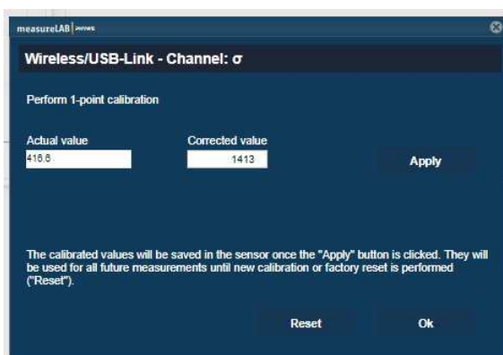
Fig. 4: Calibration of the Conductivity+ Sensor
