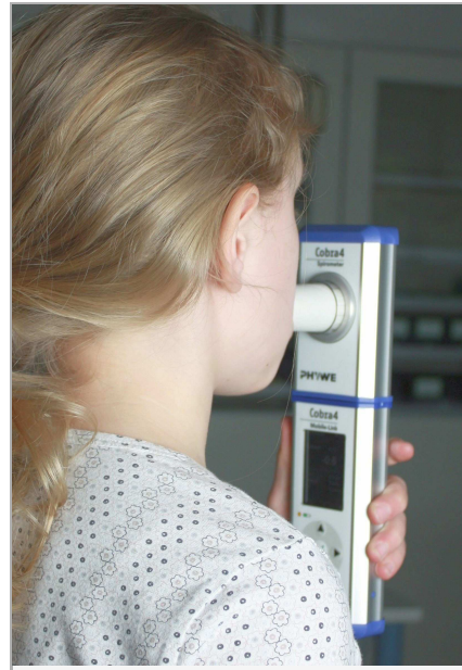
Fig. 1: Using the spirometer to determine various measured values (left: measurement by using Cobra4 Wireless/USB-Link, on the right: Cobra4 Mobile-Link)
