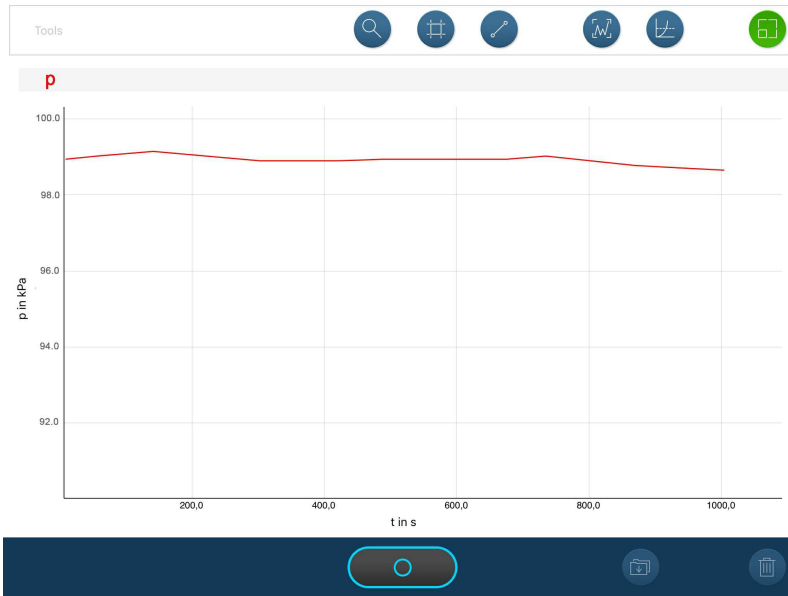
Fig. 6: Measurement result (Experiment 3) - Plant transpiration under very high air humidity
