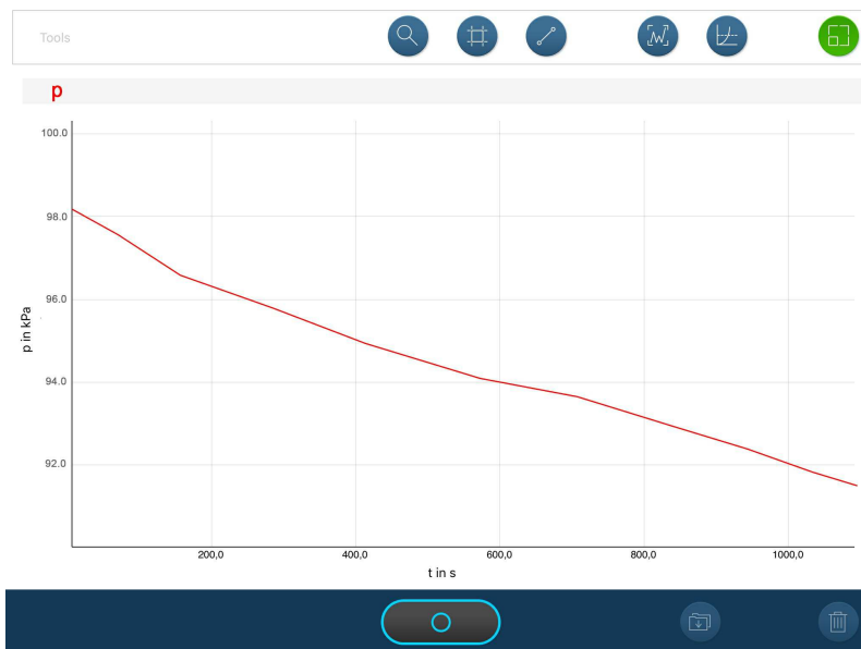
Fig. 4: Measurement result (Experiment 2b) - Plant transpiration in a flow of cold air
