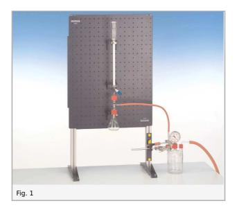
Position the clamping holders on the panel for complete experiments as shown in Fig. 2. Attach the clamp on holder for the demonstration board to the bottom of a stand leg.
