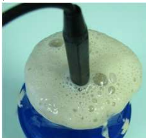
Fig. 8: Froth formation during CO 2 production
