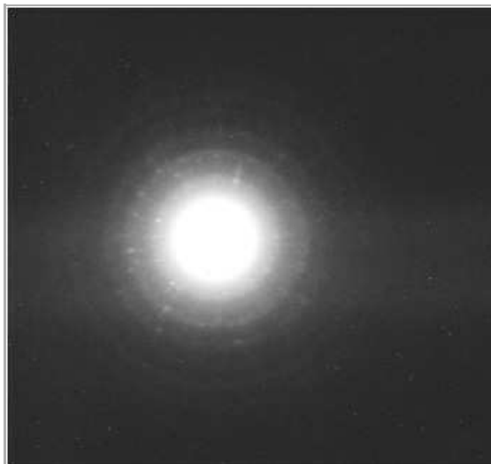
Fig. 8: Debye-Scherrer pattern of a powdered sample of NaCl. Thickness of the sample: 0.4 mm. Ex-posure time: 2.5 h. Mo X-ray tube: UA = 35 kV; IA = 1 mA
