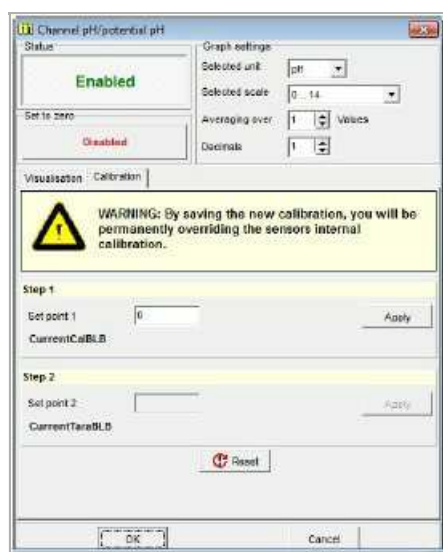
Fig. 2: Settings for the calibration mode of the sensor.
