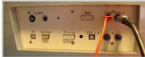
Fig. 3: Connection of the X-ray unit
