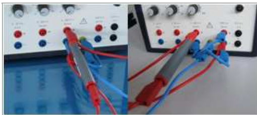
Fig. 4a: Detailed wiring at the power supply unit for measurements up to 300 V Fig. 4b: Series connection for measurement up to 600 V
