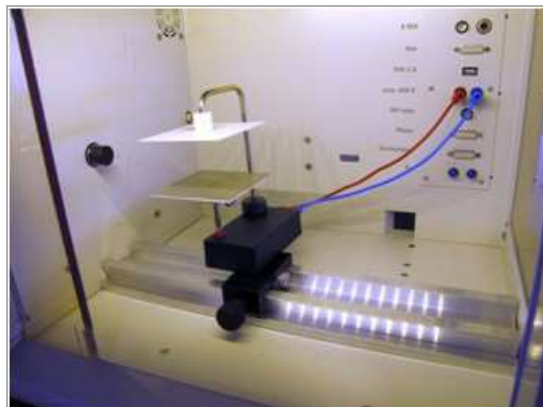
Fig. 5: Set-up and wiring of the capacitor plates inside the experiment chamber
