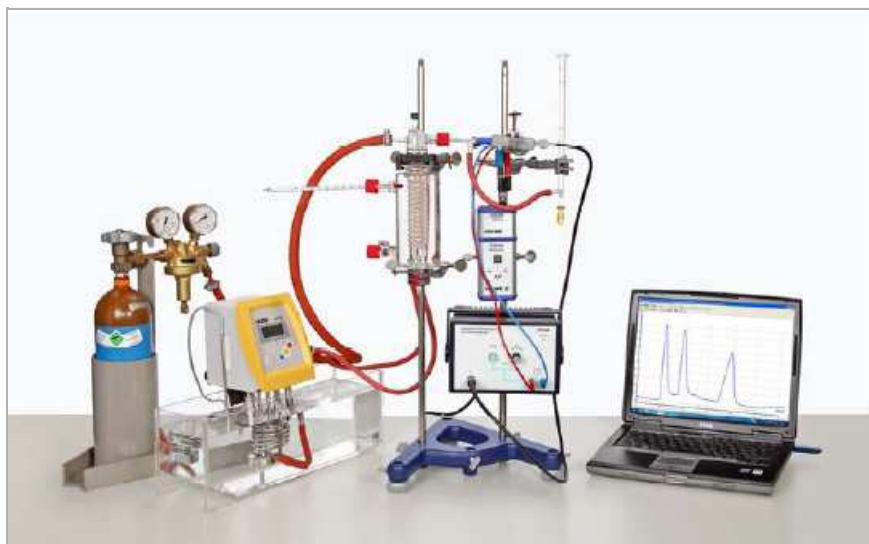
Fig. 3: Experimental set up for the gas chromatograph.
