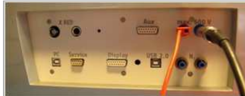
Fig. 3: Connection of the X-ray unit
