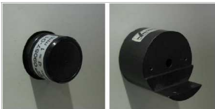
Fig. 2: Installation of diaphragm and crystal holder.
