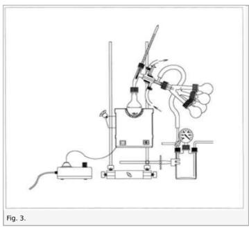
Under normal pressure, the solvent toluene distils into a 250 ml flask. Pour the remaining liquid into a 100 ml flask and equip the micro-distillation apparatus with an adapter with four flasks. Then, distil the product under the full vacuum of the vacuum pump and determine the refractive index of the purified product.
